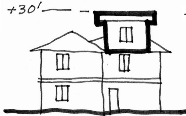
Mezzanine with flat roof
